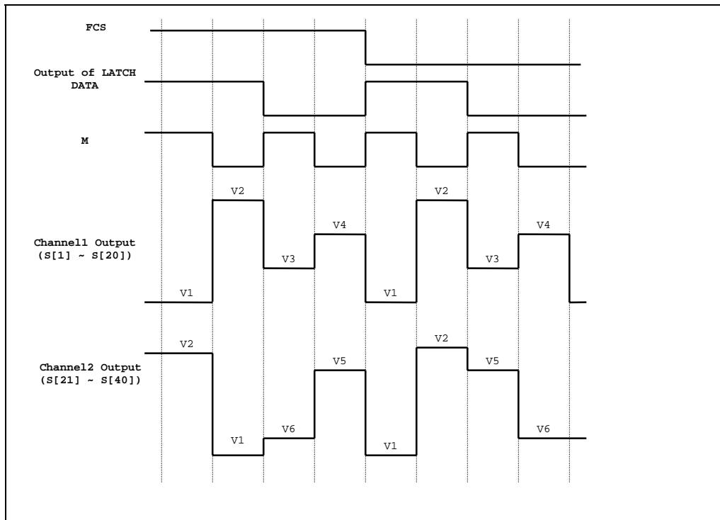
The output levels of channel1 and channel2 are decided by the combination of FCS, M, and latched data. Refer to the following table:
