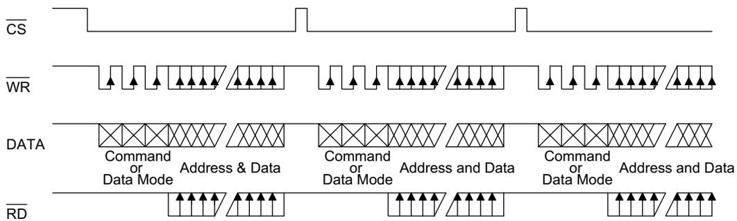
Note: It is recommended that the host controller should read in the data from the DATA line between the rising edge of the  $\overline{RD}$  line and the falling edge of the next  $\overline{RD}$  line.
