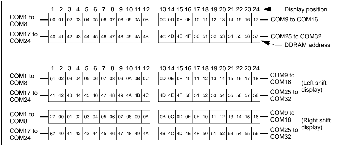
Figure 5 2-Line by 24-Character Display (5-Dot Font Width)
